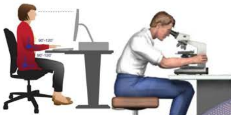
Figure 1: (A) Proper ergonomic posture when working at a desk or office environment (PanadoINZ); (B) Example of a typical posture when using a microscope (MicroscopyU)
