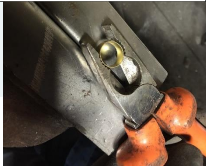
Stressing the brass rings with pliers
