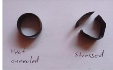
Heat annealed and stressed brass rings after 10 Days in ammonia
