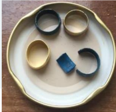
Severe corrosion, extensive pitting, some edge erosion. Pronounced corrosion, some pitting, some edge erosion.
