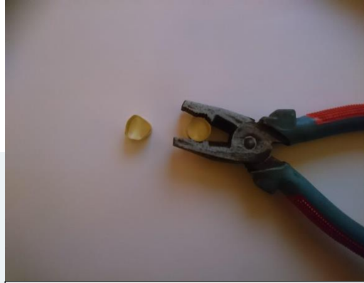
Stressing the brass rings with pliers
